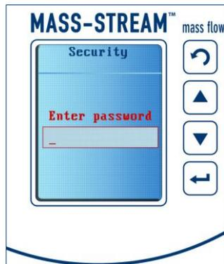
A password upon delivery protects the device from unauthorized operation and data entry via the local operator buttons. The factory settings for the password are „abc“ plus 5 blanks. **Enter** activates the screen and the password is entered with **Up**, **Down**, and **Enter**.
