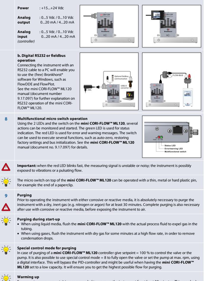
For accurate measurement, it is recommended to warm up the instrument for at least 30 minutes. This can also be done while purging or flushing.
