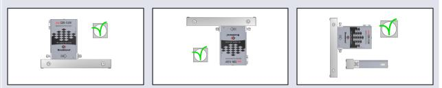
e. Mounting position when using mini CORI-FLOW<sup>™</sup> ML120 with external valve with purge connector For the mini CORI-FLOW<sup>™</sup> ML120 series instruments with external liquid valve with a purge connector, the mounting position can be critical for a good quality of de-gassing.
